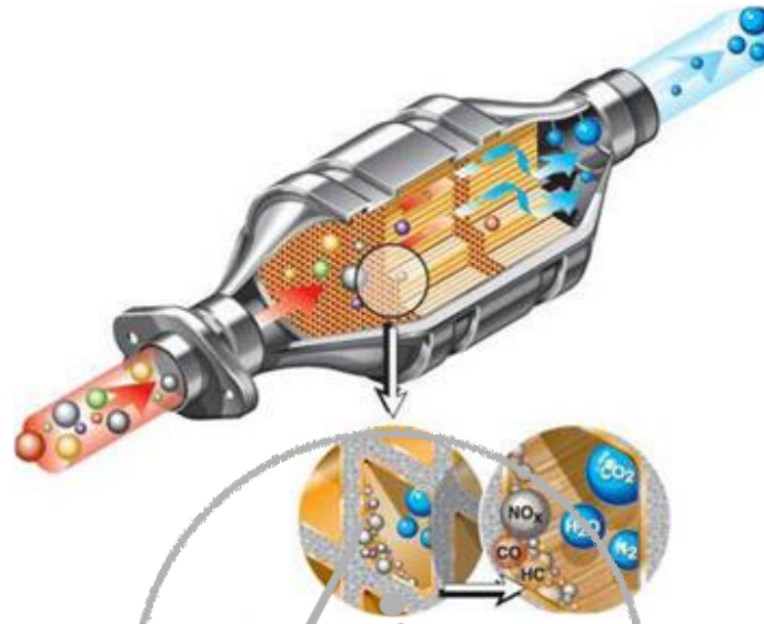
Figure 2: Catalytic Converter Working
